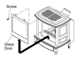
Figure 52 - Removing Glass Door from Burner System
